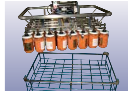
Task : Bottle (Food) Weight : App. 20Kg. Lifting Method : Suction and release
