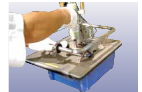
Task : Product packaging Weight : App. 20Kg. Lifting Method : Vacuum pump suction system Type of Lifting Tool : US339-A2
