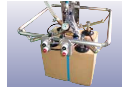
Task : Cardboard box Weight : App. 25Kg. Lifting Method : Vacuum pump suction system Type of Lifting Tool : US178-A1B
