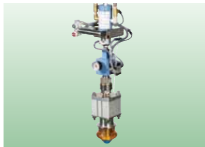
Clamping from the inside
